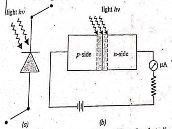
V-I characteristics of photodiode: When the photodiode is reverse biased with a voltage less than the breakdown voltage, and no light is incident on it (junction) then a small reverse saturated current flows through the junction. This current is due to thermally generated electron holepairs and is called dark current.
